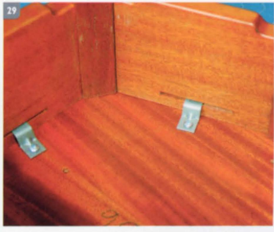
Arm-R-Seal satin finish. The Arm-R-Seal is a wipe-on/wipe-off polyurethane finish. Apply about 4-5 coats to the base and about 5-7 coats to the top. Wipe the Arm-R-Seal off thoroughly after each coat. To avoid runs use an air nozzle to blow out the excess finish from corners and crevices.
