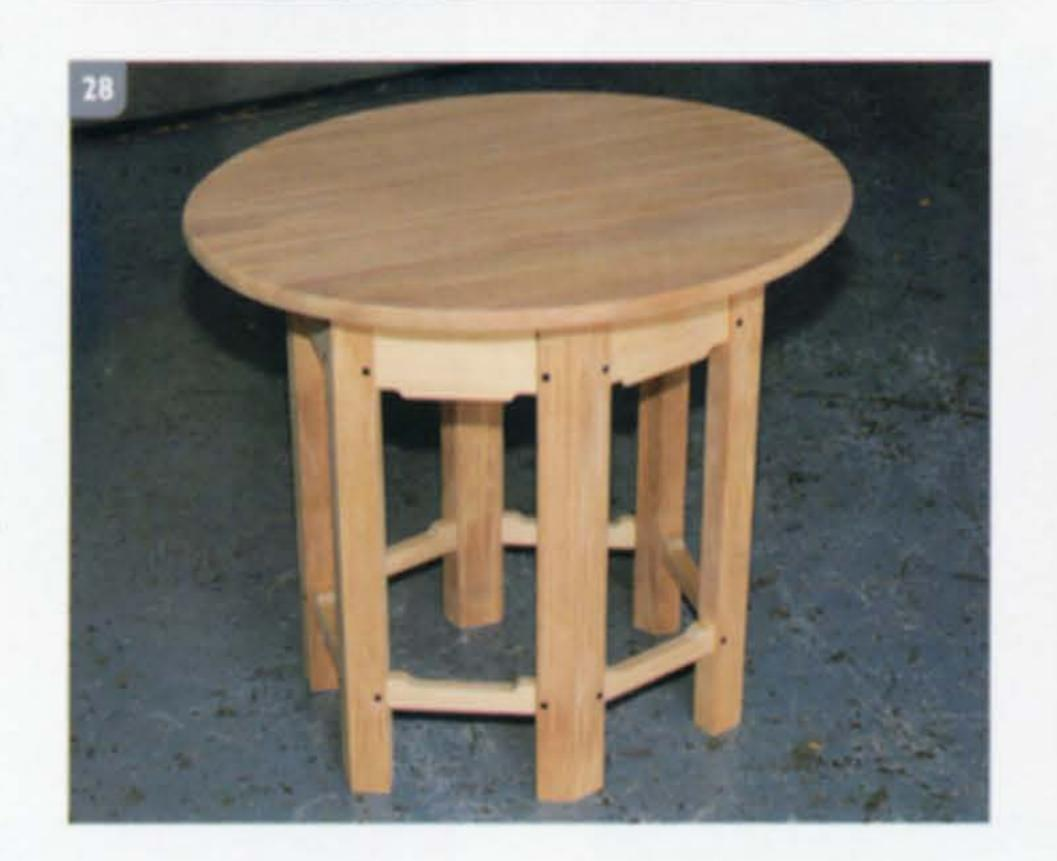
thoroughly dry, knock down the raised fibers by lightly sanding with 320-grit (28).
